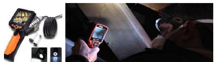
Figure 17: Endoscope/borescope for inspection of narrow space
